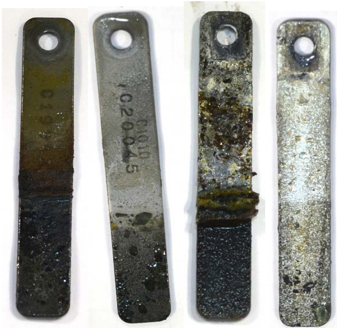
Steel Coupon Compressed Air
